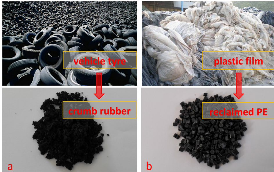
Fig. 1. Morphology of the additives before and after reclaim (a) crumb rubber and (b) reclaimed PE.
